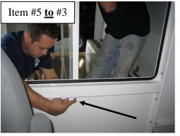
Loosely bolt **Center Divider** to **Front Bulkhead**
